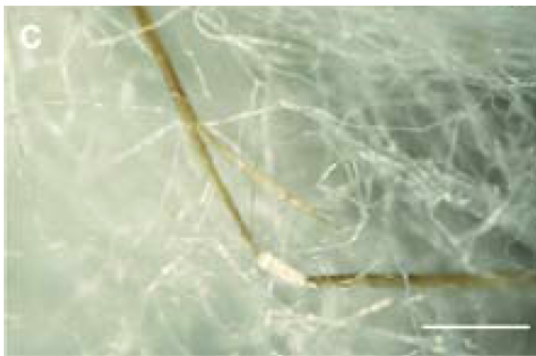
Figure 3.12: Impurities in cotton: (a) fibre entanglement (neps), (b) seedcoat fragment with other fibres attached to it, (c) unidentified non-seed impurity (bar= 0.5 mm)
